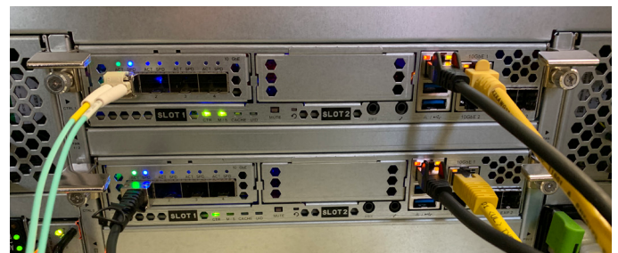
Figure 3: Two 10GB/s SFP+ connections (left) together with the 10GbE LAN (yellow cables) and 1GbE management (black cables) ports (right).
